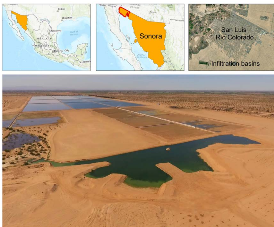
Figure 1. Location of San Luis Río Colorado Infiltration Basin Artificial Recharge (IBAR) system in Mexico (top) and an aerial photo of the IBAR (bottom). Basins are operated alternately (ie Soil Aquifer Treatment) with drying times between to assist treatment and to help manage clogging. Source: Own elaboration; Photo © Jorge Ramirez Hernandez
